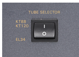
A side-mounted rocker switch changes bias to suit EL34s, KT88s and even KT150s PrimaLuna say.
